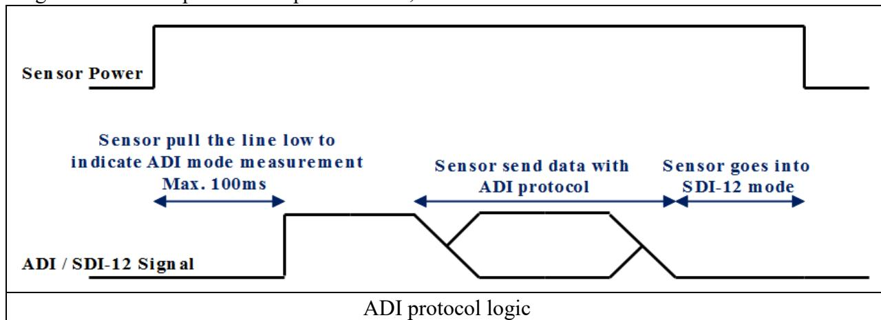
ADI interface is TTL compatible standard(0-3.6V),protocol data stream is encoded in ASCII,Baudrate 1200bps,None parity,8 data bits,1 stop bit.The sensor enter into SDI-12 standby mode after the ADI output.You'll need to re power up the sensor again for another ADI output.ADI interface transmission bit diagram is as following.
